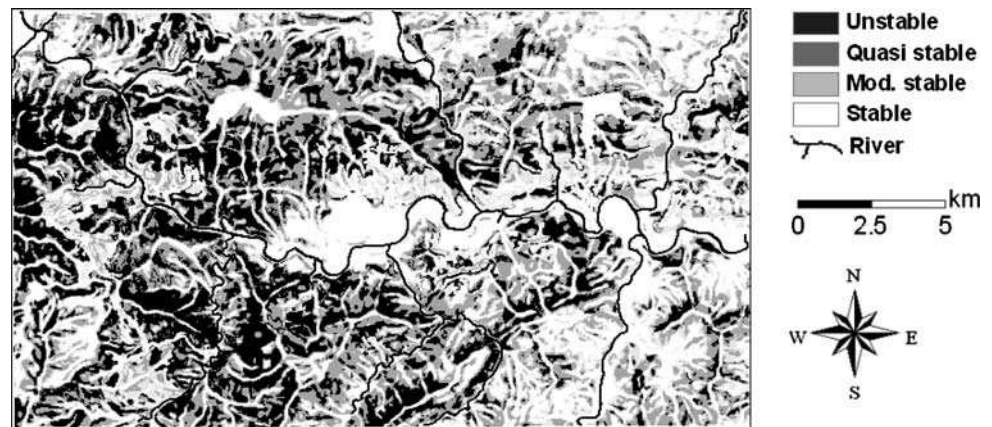
Fig. 9 Safety factor map for saturated soil conditions
